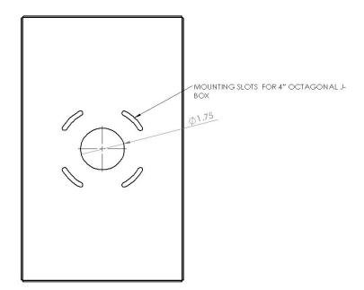
**NOTE:** Verify the mounting hole dimensions before installing the fixture.
