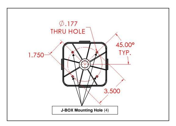
**NOTE:** Fixture is to be centered over junction box and mounted to the wall using (8-32 screws) from j-box.
