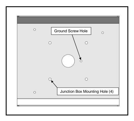
**NOTE:** Fixture is to be mounted to the junction box using 8-32 x .75 screws
