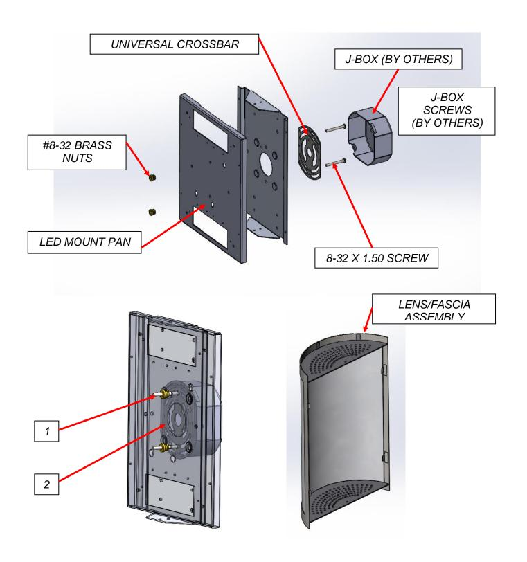
NOTE: Fixture is to be mounted to the junction box using supplied mounting hardware kit.
