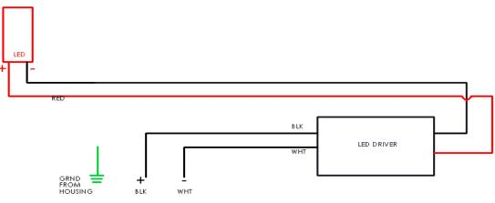
ONE DRIVER ONE MODULE WIRING DIAGRAM
