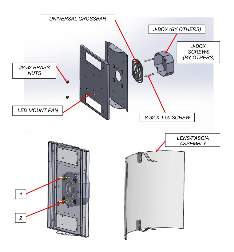
NOTE: Fixture is to be mounted to the junction box using supplied mounting hardware kit.
