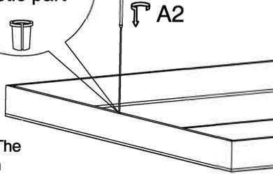
Attention :This fitting is multi-wire load-bearing. The force of each suspension wire must be balanced during installation.
