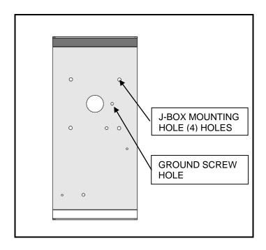
**NOTE:** Fixture is to be mounted to the junction box using 8-32 x .75 screws (supplied by others).
