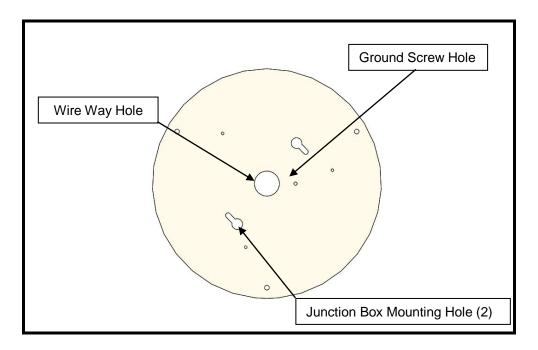
NOTE: Fixture is to be mounted to the junction box using 8-32 x .75 screws
