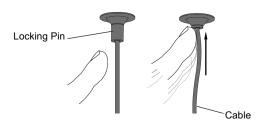
The length of the cable is adjustable. To determine the proper length of the fixture, hold the fixture canopy up against the outlet box in the ceiling and adjust the cable.
