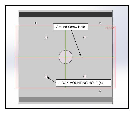
**NOTE:** Fixture is to be mounted to the junction box using 8-32 x .75 screws
