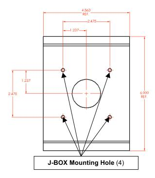
**NOTE:** Fixture is to be centered over junction box and mounted to the wall using (8-32 screws) from j-box.
