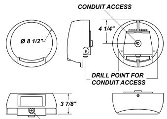
PHOTOCELL OR CONDUIT ACCESS LOCATION
