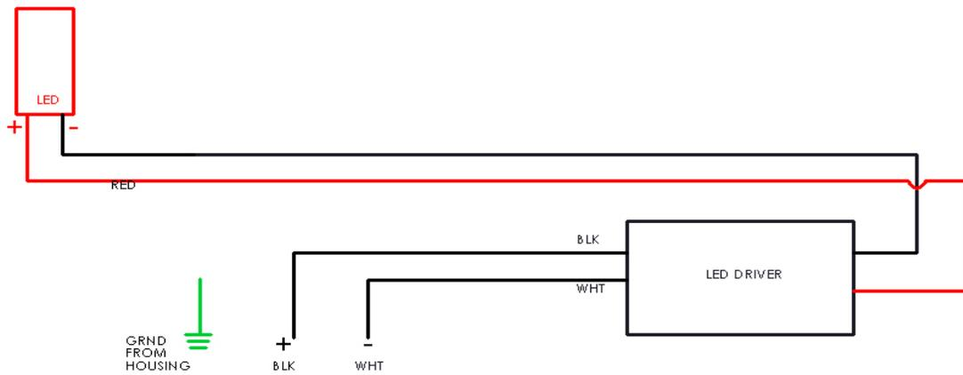
**ONE DRIVER ONE MODULE WIRING DIAGRAM**
