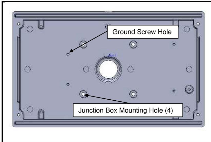
**NOTE:** Fixture is to be mounted to the junction box using 8-32 x .75 screws
