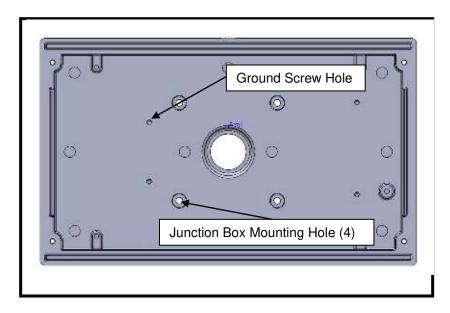
**NOTE:** Fixture is to be mounted to the junction box using 8-32 x .75 screws
